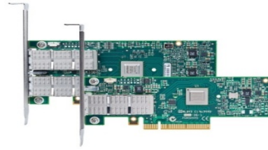
High Performance Interconnects – InfiniBand <1 \mu s latency, >100 Gbps Bandwidth
