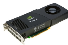
Accelerators / Coprocessors high compute density, high performance/watt >1 Tflop/s DP on a chip
