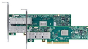
High Performance Interconnects - InfiniBand <1us latency, >100 Gbps Bandwidth
